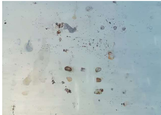
Image no. 3 The results of some tested samples of Patina recipes with two and four ingredients on Stainless Steel Metal (2026).
