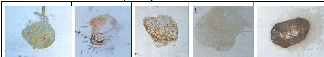
Image no. 4 The detail images of few tested samples of Patina recipes with two and four ingredients on Stainless Steel Metal (2018-2026).
